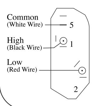
White Wire – to be connected to common terminal on motor
